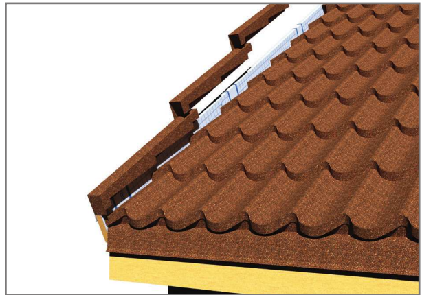
Fig 9.4.2 Gable flashing installation
