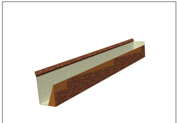
Fig 9.4.4 The flashing with glued sealant
