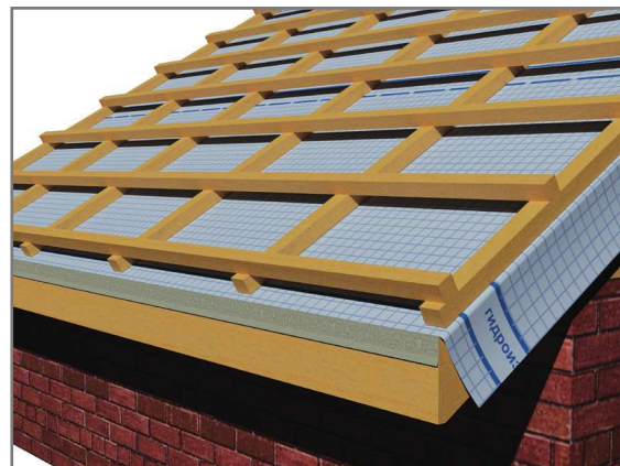
Fig 8.4.2 The roof sheathing without rainwater hooks
