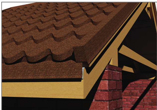
Fig 9.4.5 The gable board with ending cap installation
