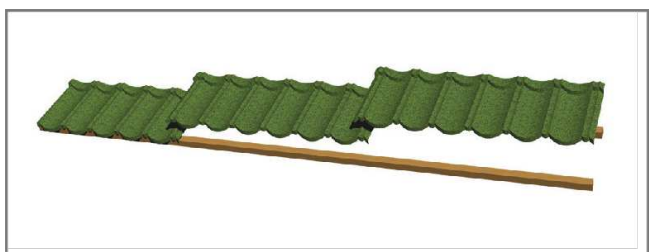
Fig 9.1.6 Overlapping the tiles from left to right
