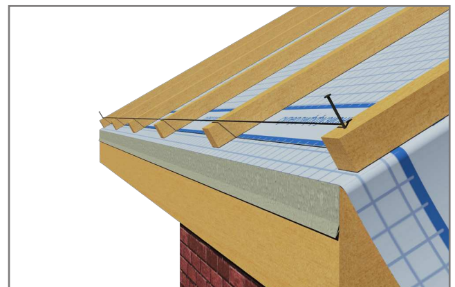
Fig 8.5.1 Marking of the intermediate points of the slope
