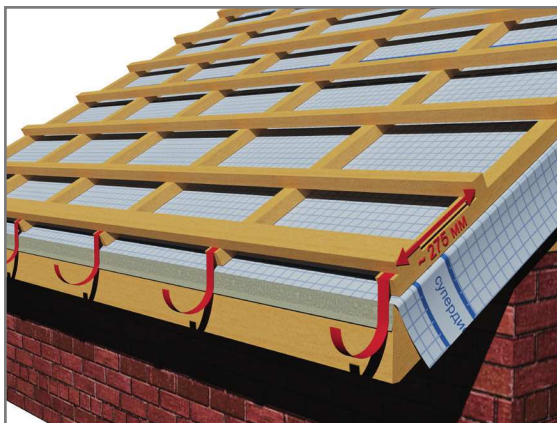
Fig 8.4.1 The roof sheathing with rainwater hooks
