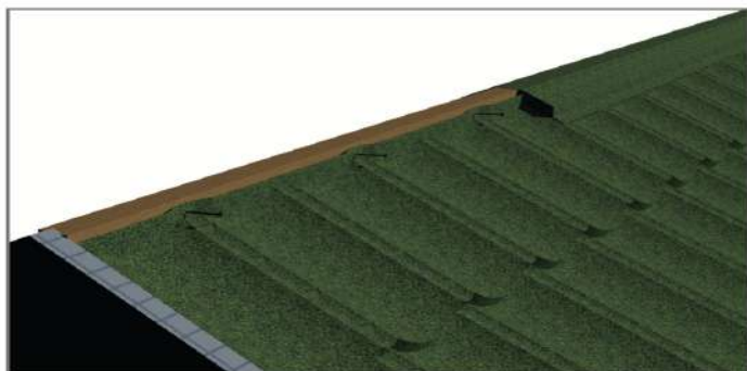
Fig 9.2.8 Tile's adjoining to the ridge batten without using the roofing tape
