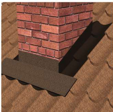
Fig 9.5.5 Side flashing installation in the lower part of adjoining node
