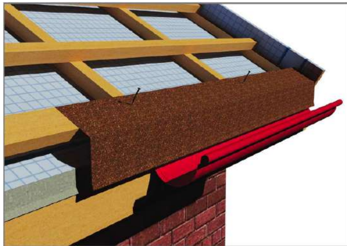
Fig 9.1.2 Big eave flashing installation
