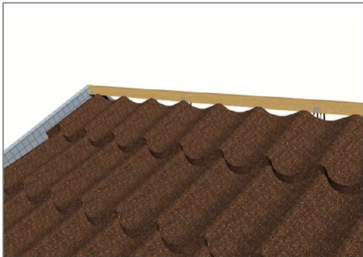
Fig 9.2.1 Tile adjoining to the ridge batten
