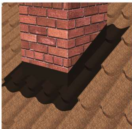
Fig 9.5.4 Gluing the roofing tape
