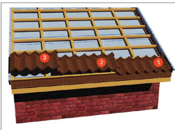
Fig 9.1.10 The installation of the first row
