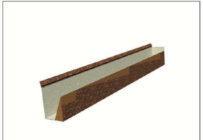
Fig 9.4.4 The flashing with glued sealant
