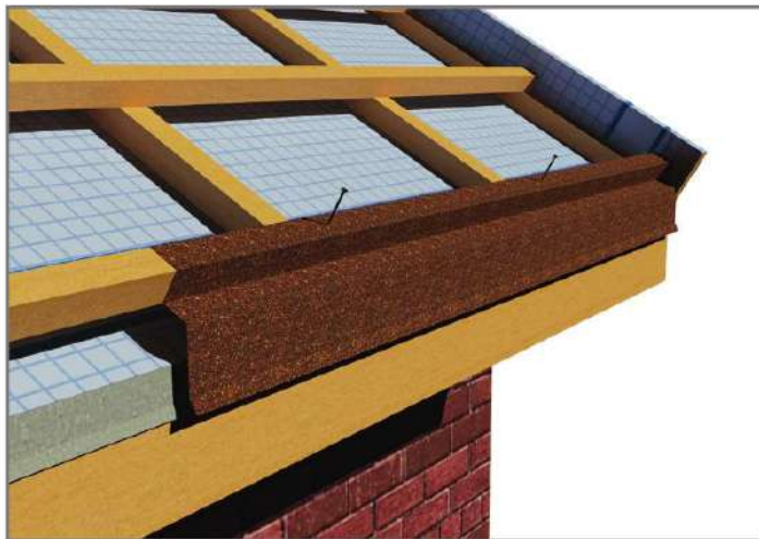
Fig 9.1.1 Small eave flashing installation
