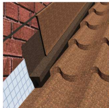
Fig 9.5.8 The adjoining of roof pitch to the wall parallel to the slope
