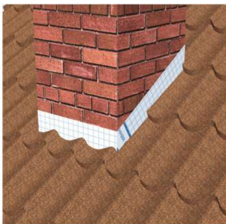
Fig 9.5.2 Tile installation in the place of adjoining
