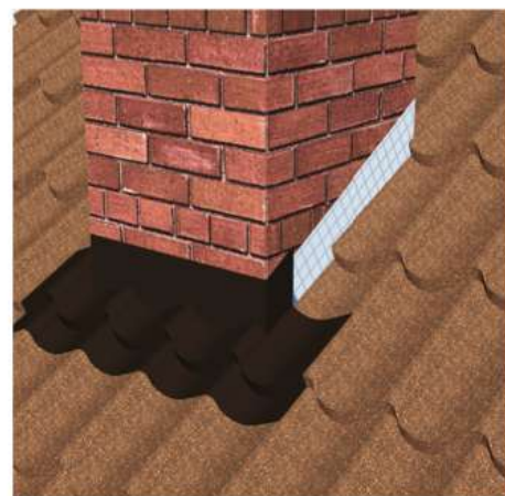
Fig 9.5.3 The roofing tape gluing in the lower part of adjoining
