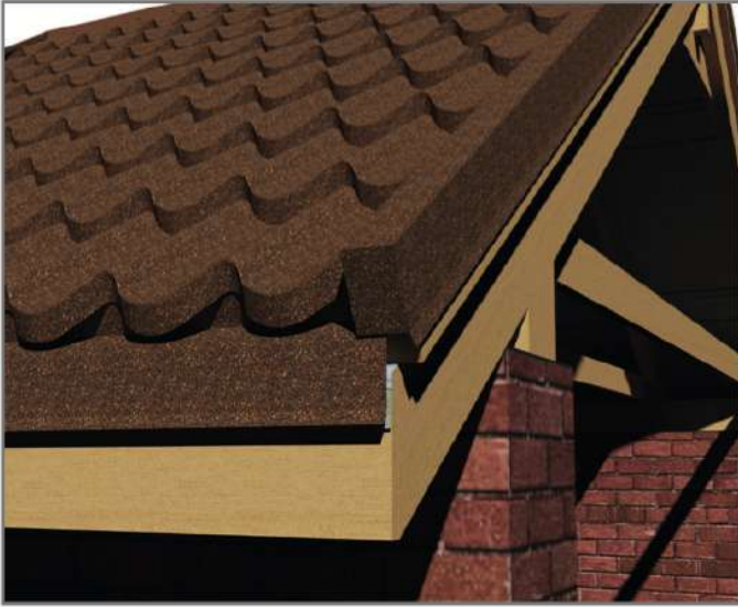
Fig 9.4.5 The gable board with ending cap installation
